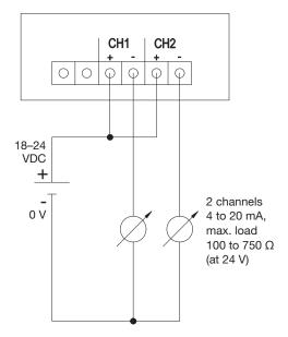
Connection plan 4-wire technology (0 to 20 mA / 4 to 20 mA / 0 to 1 V / 0 to 5 V / 0 to 10 V)
