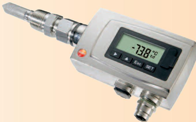
The transmitter testo 6781 was developed specially for trace humidity measurement in compressed air and in dry air (e. g. in granulate dryers). The international norm ISO 8573 categorizes seven classes of compressed air. High-performance adsorption dryers are required in order to meet the highest quality classes 1 and 2. They can be monitored by the testo 6781 down to very low dewpoints of  $-90\text{ °C}_{td}$ .
